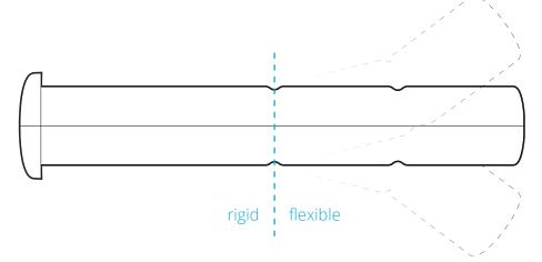
It is designed to be inserted inside the handlebar, leaving only the "head" outside.
