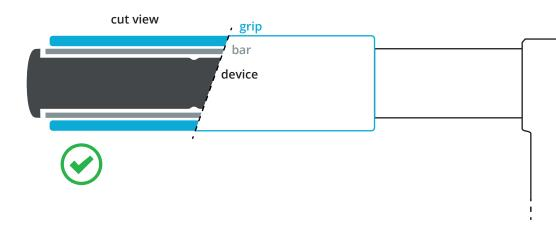
If the grip closes the bar end completely, or leaves a hole smaller than 19 mm in diameter, it is not compatible with Sherlock. You can hack your grip, given that you don't modify the product or cover its "head".
